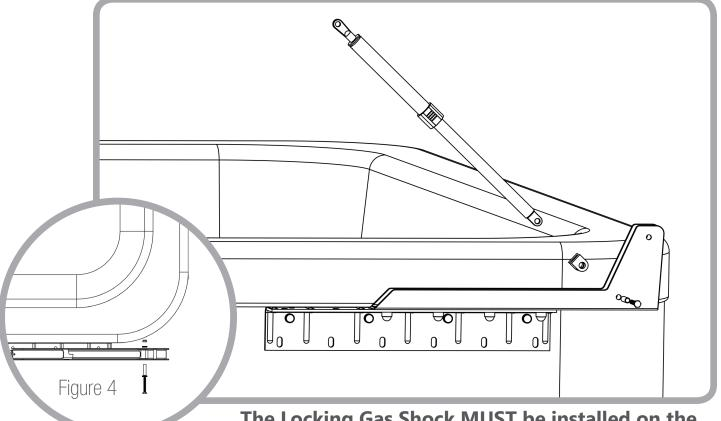
The Locking Gas Shock MUST be installed on the side of the spa where you will operate the lift.
